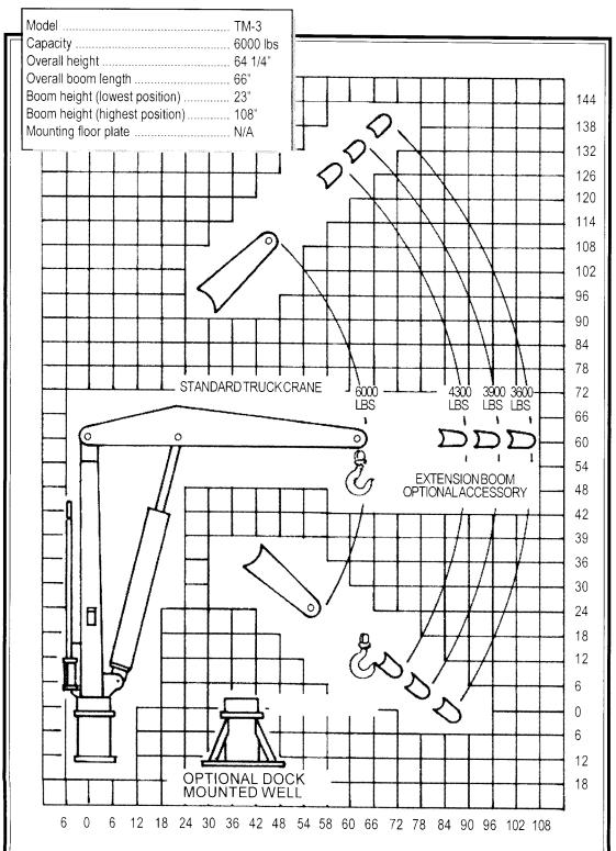
PUMPING CYCLES needed to raise boom through full travel; 35 with crane set for speed and 60 for crane set for power.
